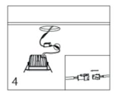
Connect the light to the driver via the plug.
