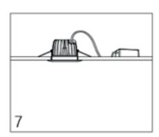
Release the springs, it will lock the lamp on the ceiling.
