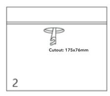
Cut out a hole in the ceiling at a certain diameter given in the box label.
