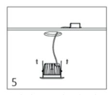
Put the driver onto the ceiling, then pull the springs into vertical state.
