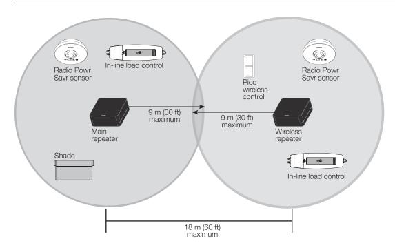
All devices must be located within 9 m (30 ft) of a repeater. The range can be extended with up to four RA2 Select wireless repeaters ( $L\underline{x}$ -REPPRO).
